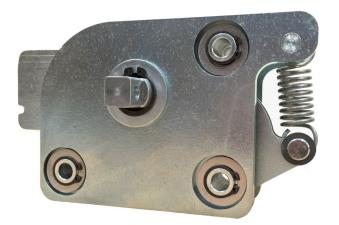
This heavy duty cam lock module is designed to be located in high stress areas and used as a primary mechanism for securing personnel doors, rear doors, hatches and windows or as a secondary mechanism in conjunction with a primary door latch. Providing additional strength and security, it can be used singularly or in multiples and can be operated and controlled via rods or cables from a central release such as TriMark's 010-1000 Inside Release Handle.
